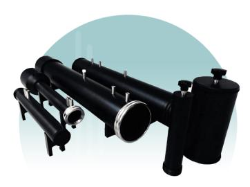
The Impedance tube (also known as Kundt Tube) measures, calculates and lets the user analyze Parameters like the Sound normal incidence absorption(Absorption Coefficient, Reflection Coefficient, Impedance, Admittance) and Sound Transmission/sound insulation (Transmission Loss, Transmission Coefficient) of the material under test.
